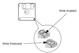
Figure 4-5. Floppy Disk Write Protect
